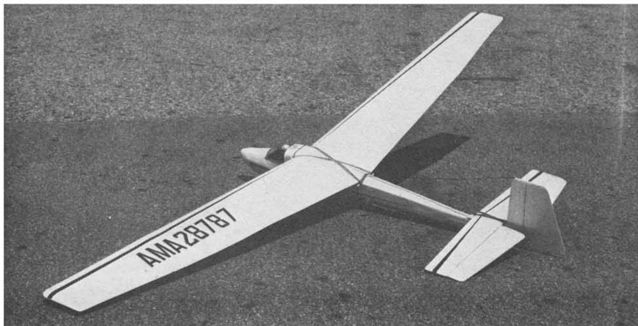
Dale Willoughby's "Big Sailer" under construction. A modified Cumulus Zeus fuselage with Eppler E-385 airfoil and 1200 square inches of area. The glide proved slow and majestic with a gross weight of 9 lbs. It died gracefully in Norway attempting to set a World Record in Duration.
